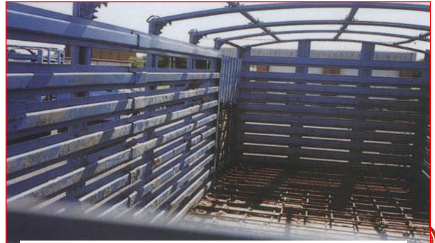
Cross slating of cattle truck floor to prevent slipping
