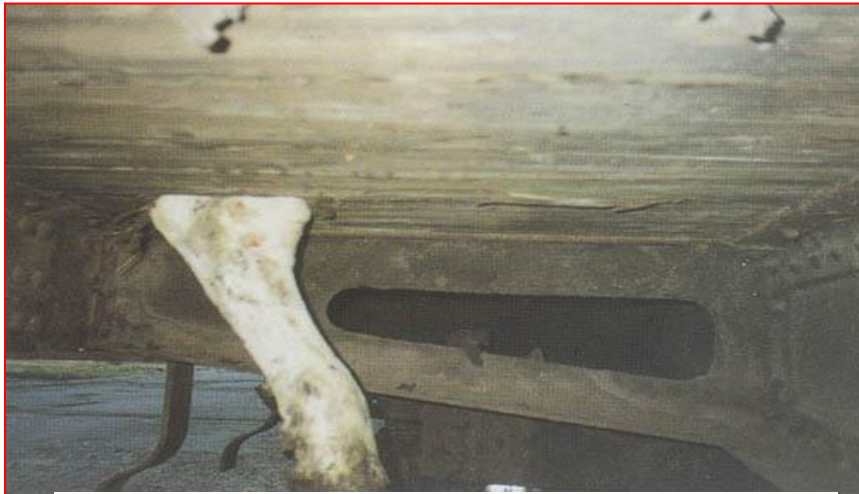
Cattle leg protruding through broken truck floor
